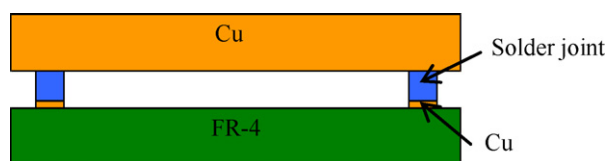
Fig. 1. Schematic cross-sectional geometry of the solder/Cu samples.
